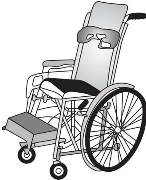
Fig. 5.5: Modified wheel chair with head and feet supports for cerebral palsied child
